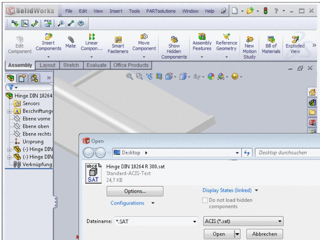
Open exported part in the CAD system (here exemplified SolidWorks)
